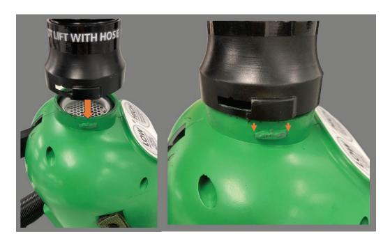
2. Firmly gripping the plastic neck of the Hose Attachment, rotate the Hose Attachment counterclockwise until the piece of green plastic protruding from the neck of the pump is completely revealed and resting in the open slot on the neck of the Hose Attachment.
