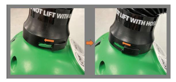
2. Firmly gripping the plastic neck of the Hose Attachment, pull up on the attachment until fully separated from the neck of the pump.
